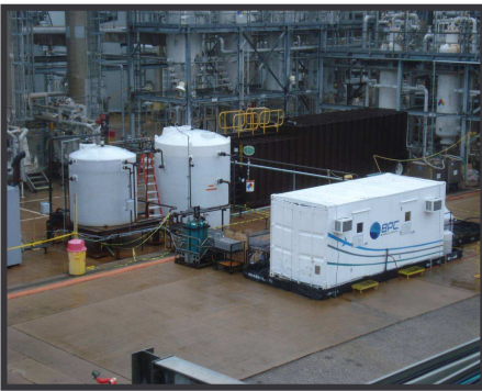
Figure 1: BPC-ACT™ pilot system for treating bilge water
