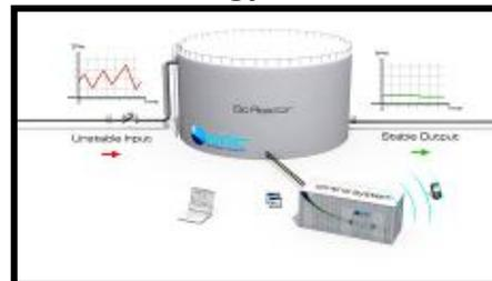
**Figure 3: A schematic description of BPC-ACT™ technology: The bioreactor receives a highly contaminated (and sometimes fluctuating) inlet, and releases a low and stable outlet. The control unit continuously monitors the process.**
