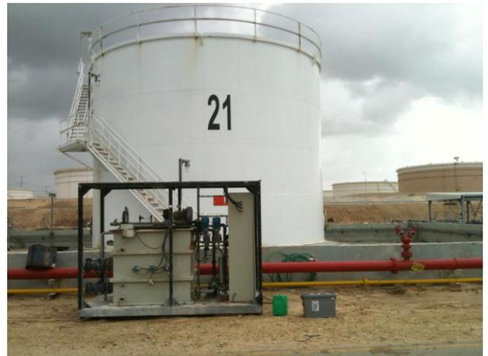
In the next step, BPC placed an auto-starter unit in which the bacterial cells were cultivated to reach a certain concentration. When a satisfying concentration level was achieved, the bacteria were introduced into the water in the storage tank/bioreactor. The biodegradation was performed within the tank in batch mode for a duration of one week. By the end of the project, the water was transported to a nearby water treatment site for further treatment and discharge.
